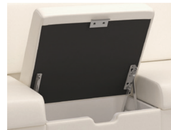
SEAT MODULE WITH STORAGE Available in left, center and right seat positions. Storage features a cleanable interior surface with a vented plastic bottom with a clean-out for debris and liquids. The spring-assisted, stainless steel mechanism holds the seat in the upright position to provide safe access.
